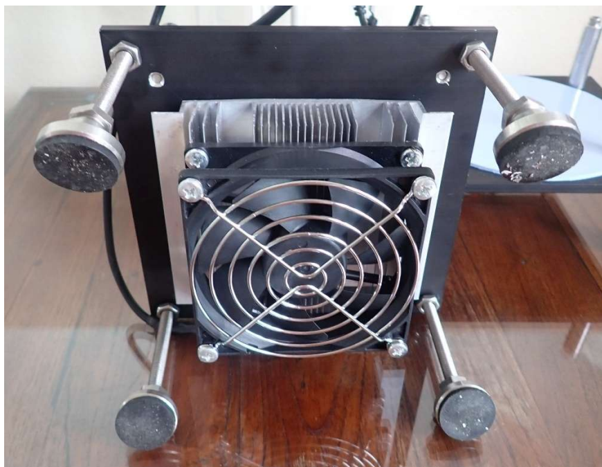
Peltier Cooler Assembly on the Underside of the Inverse Solubility Base
