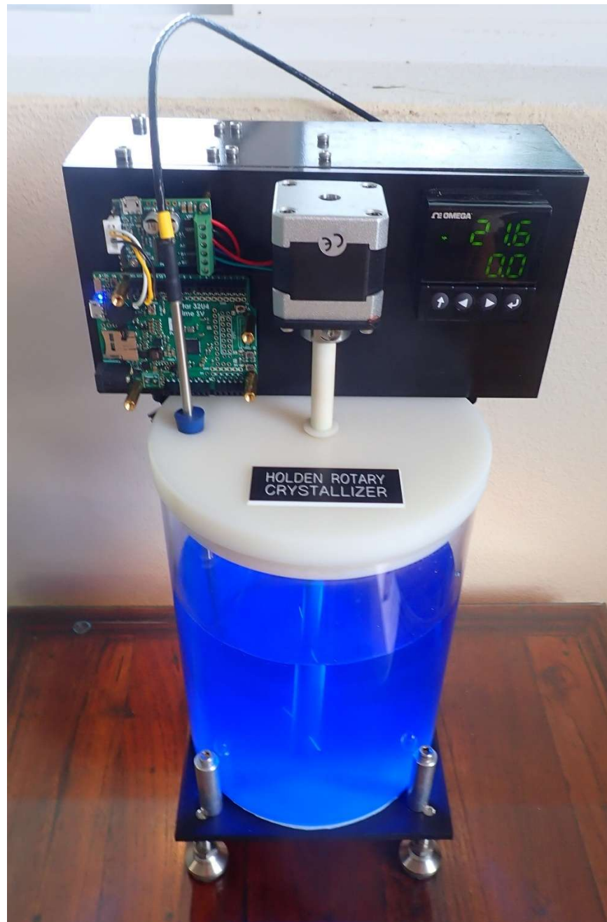
Rotary Crystallizer with Copper Sulfate Solution
