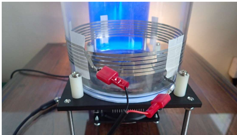
Nichrome heating element, crimp connections, and glass cloth tape
